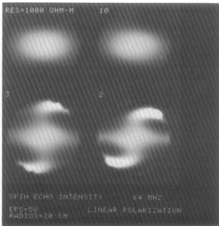
FIG. 3. Simulations of rf inhomogeneity for linear polarization as resistivity is varied. In lossless case pattern is symmetric about field. At lower resistivity, eddy currents cause quadrupole artifacts.
