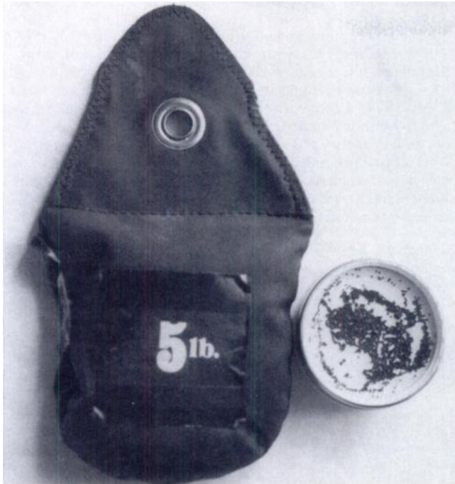
Damaged metal-filled 5-lb (2.25 kg) "sandbag" (resealed) and the cup containing ferromagnetic pellets retrieved from the severely damaged MR unit.
