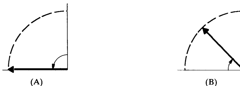
Figure 1. (A) Correct representation of a net magnetization vector being tipped during a pulse. (B) INCORRECT representation of a net magnetization vector relaxing in the absence of radiation damping.
